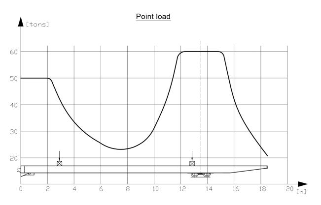
Point loads on the platform to be placed or transferred using transversal supports to the longitudinal beams
