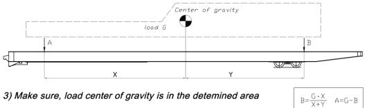
4) Loads A and B shall not exceed the limit line in above diagram
